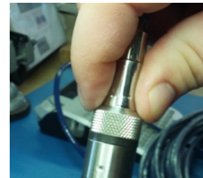
Properly completed—black ring uncompressed
