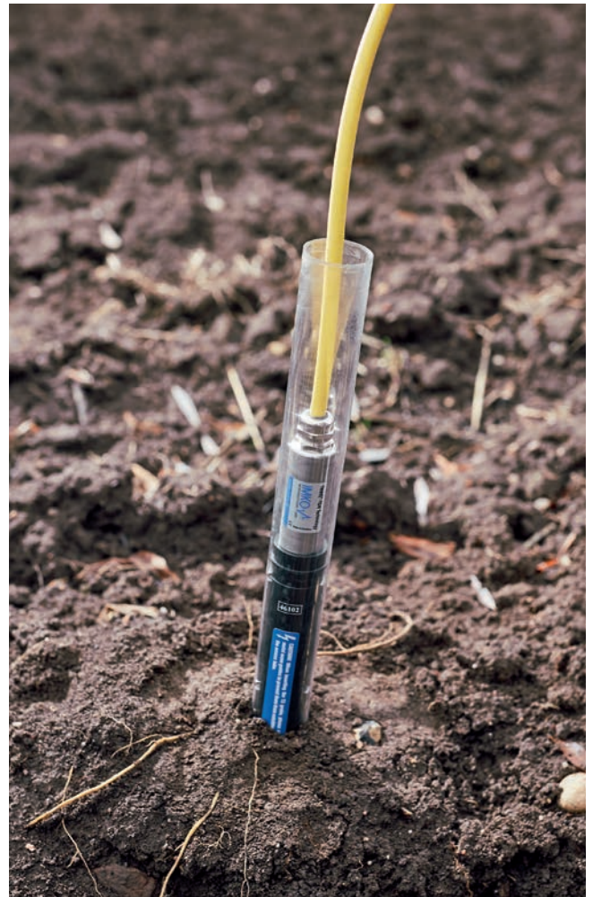
Example of the utilization of an IPH2 in the undisturbed subsoil - the special polycarbonate tube is displayed in the center
