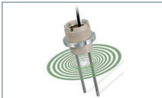
TRIME GR probe with electromagnetic field
