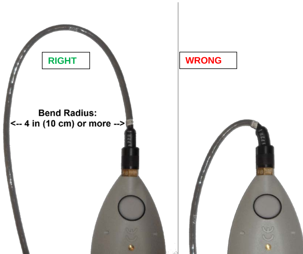
Figure 72. Cable Bend Radius
