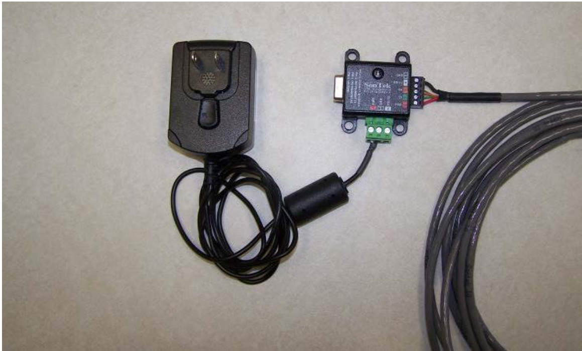
Figure 17. Connecting the Power Supply to Cable Adaptor
