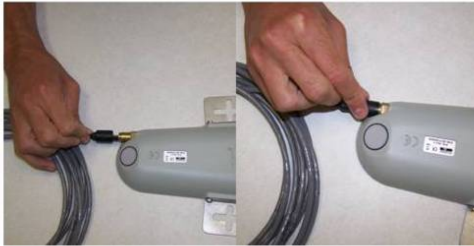
Figure 15. Connecting IQ to Power and Communications Cable
