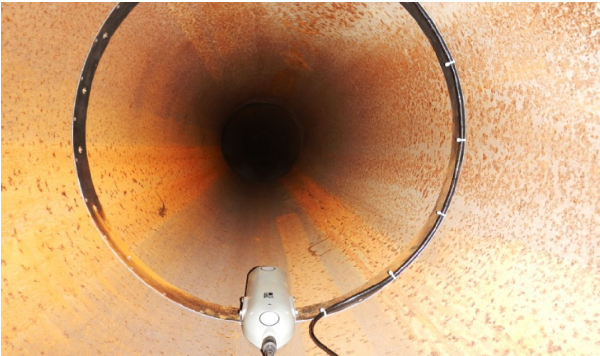
Figure 14 . SonTek-IQ Pipe Installed with SonTek Pipe Ring
