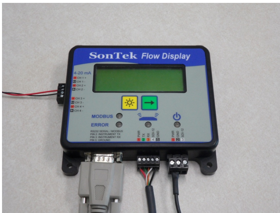
Figure 19. Flow Display Connections
