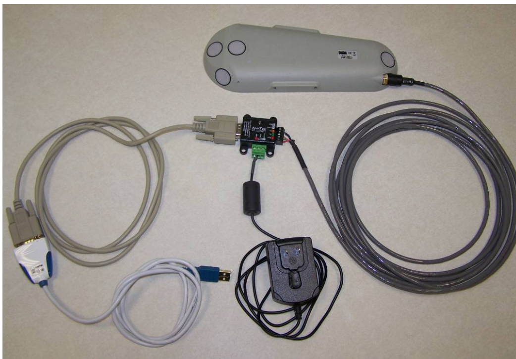
Figure 18. Connecting the USB-Serial Adaptor to Cable Adaptor
