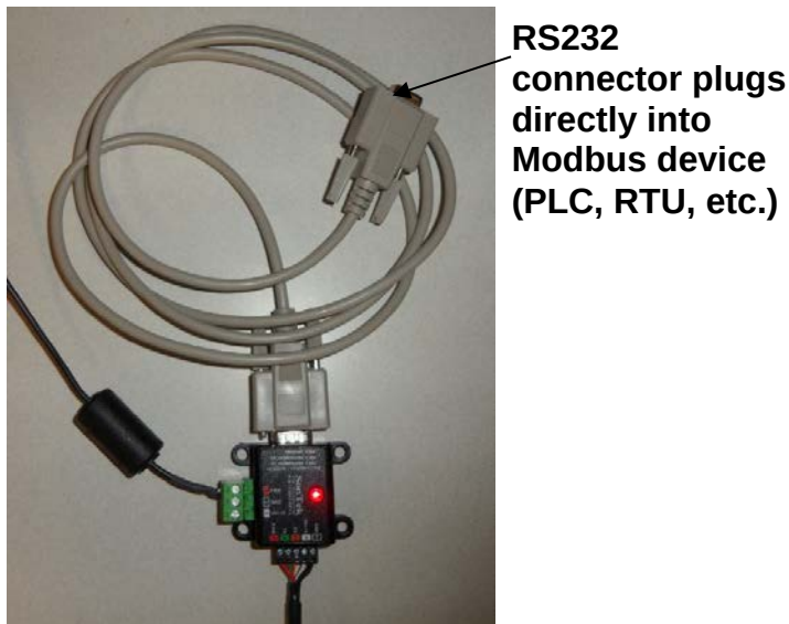
Figure 100. Modbus Connection with RS232 Cable
