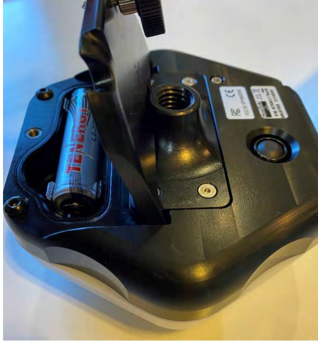
Figure 11. SonTek Base Station with Battery
