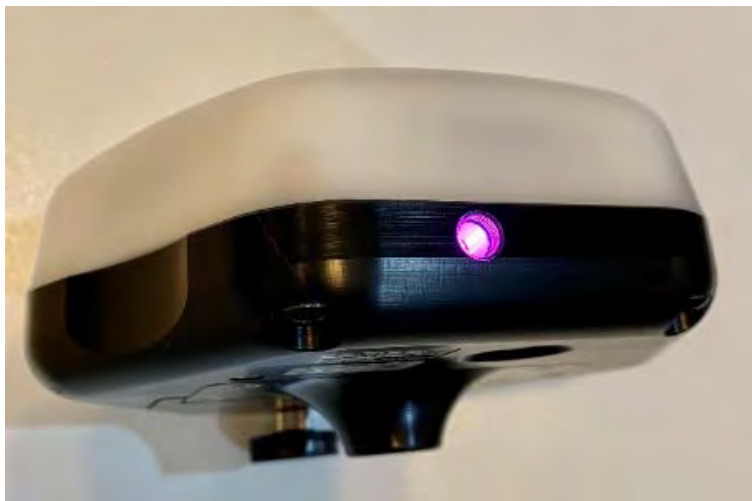
Figure 12. RTK Base Station Antenna with Indicator Light
